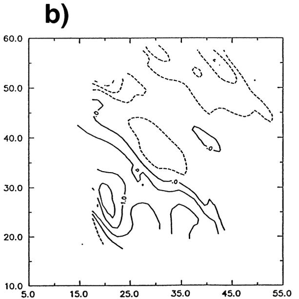
FIG. 10. The 2239 UTC low-level ( $z = 2.25$  km) perturbation azimuthal divergence ( $10^{-3} \text{ s}^{-1}$ ) for (a) the dual-Doppler analysis and (b) the retrieval performed in the mean wind reference frame. The contour interval is  $0.5 \times 10^{-3} \text{ s}^{-1}$ . Grid distances and radar location are as in Fig. 5.
