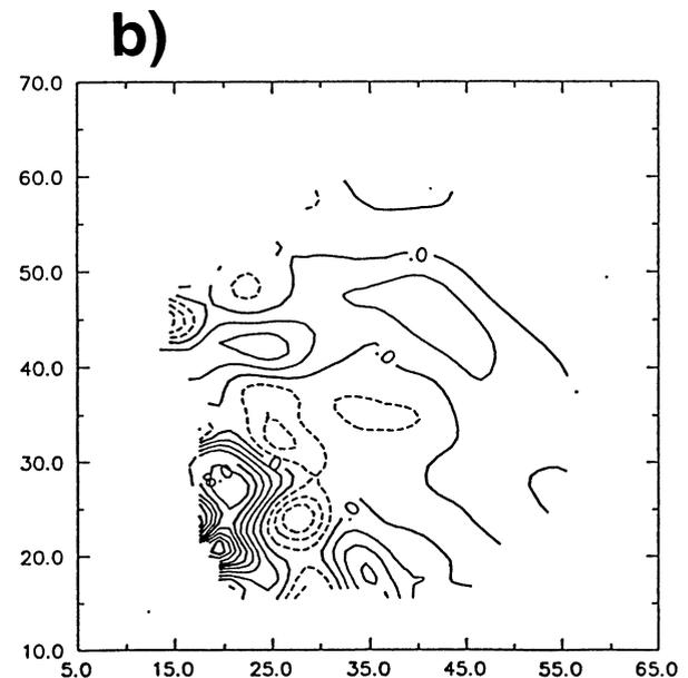
FIG. 13. The 2239 UTC retrieved fields from the simplified velocity retrieval. (a) Low-level ( $z = 2.25 \text{ km}$ ) azimuthal velocity and (b) midlevel ( $z = 6.25 \text{ km}$ ) vertical velocity. Azimuthal and vertical velocity are contoured every  $2 \text{ m s}^{-1}$ . Grid distances and radar location are as in Fig. 5.
