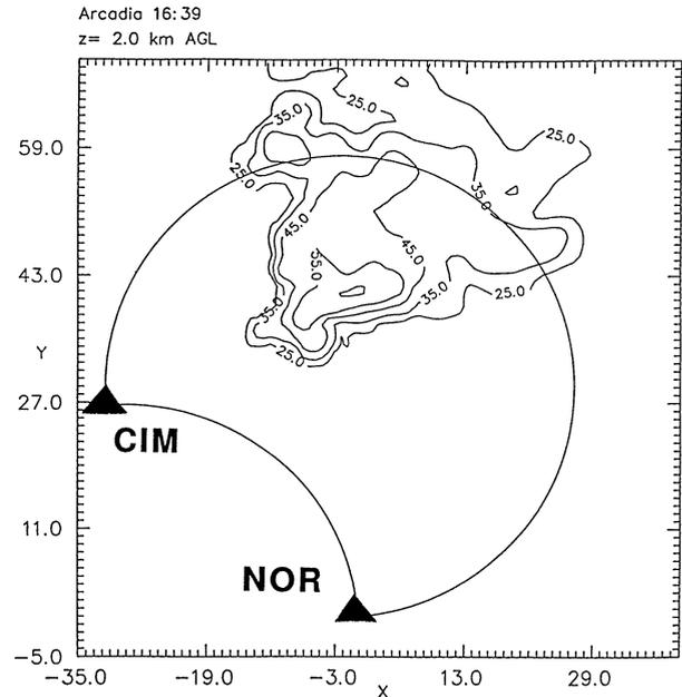
FIG. 2. Locations of the Cimarron, OK (CIM), and Norman, OK, (NOR) radar sites and the crescent-shaped dual-Doppler lobe relative to the Arcadia storm at 2239 UTC 17 May 1981. Contours are radar reflectivity in 10-dBZ increments (starting with 25 dBZ). The grid origin is collocated with NOR and  $x$  and  $y$  distances are in km.
