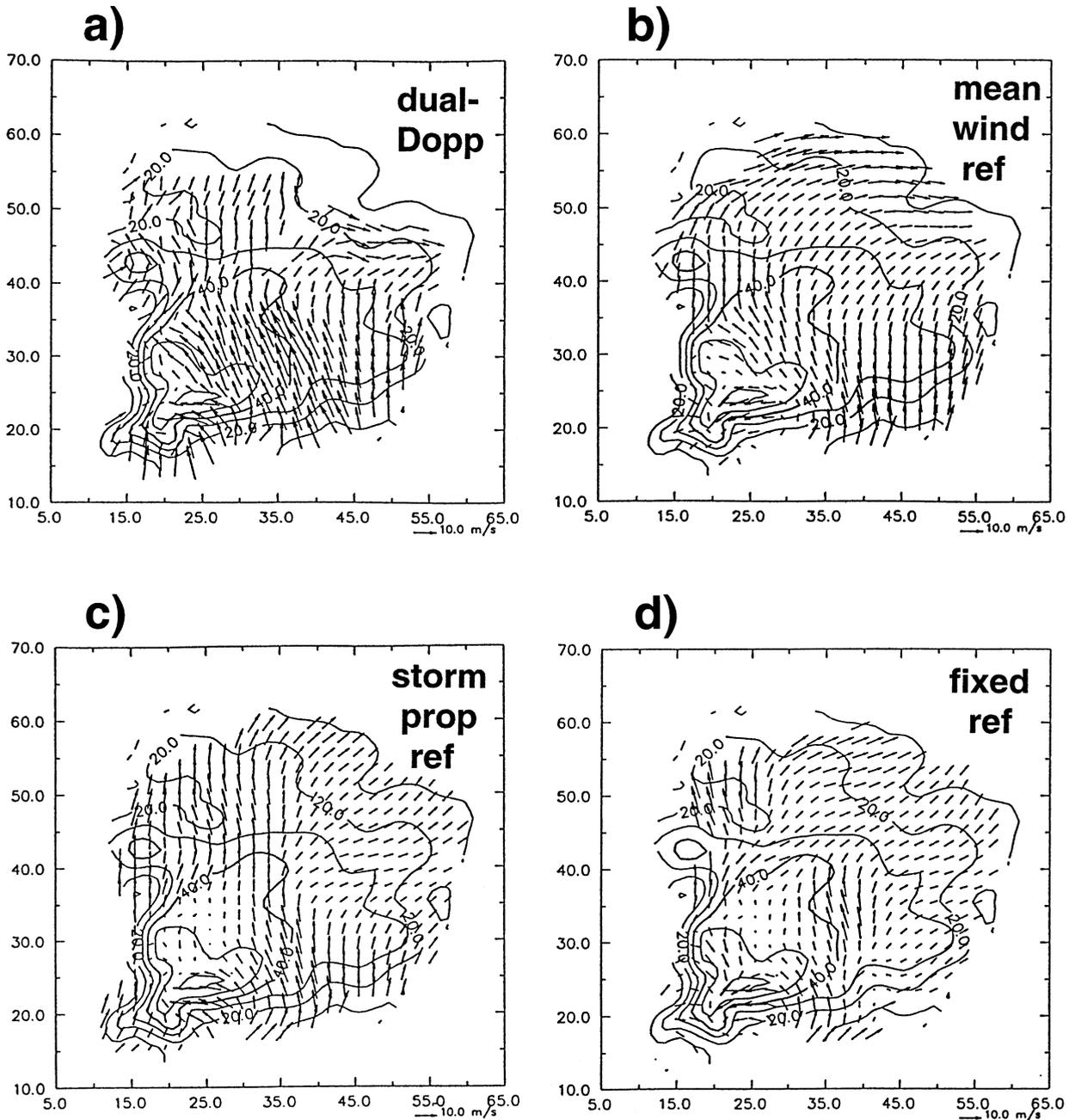
FIG. 5. The 2239 UTC low-level ( $z = 2.25$  km) reflectivity and storm-relative horizontal vectors for (a) the dual-Doppler analysis, and the retrieval performed in (b) the mean wind reference frame, (c) the storm propagation reference frame, and (d) the fixed reference frame. Reflectivity is contoured every 10 dBZ. Grid distances are in km and CIM (input) is located at  $x = -5$ ,  $y = 10$ .
